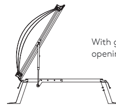
With gas spring fitting, chain drive and ladder bracket
